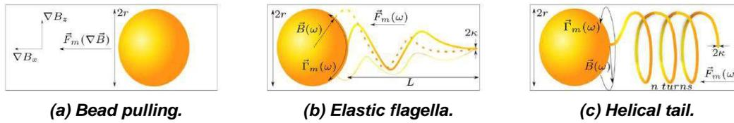
Figure 2: Different magnetic microrobots propulsion designs. (a) Bead pulling: control input is the magnetic gradient [2, 3, 4]. (b) Elastic flagella: control inputs are the time-average magnetic field direction and the frequency [5, 6]. (c) Helical tail: control inputs are the magnetic torque direction and the frequency [7, 8].
