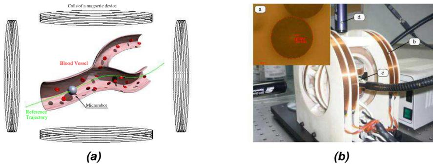
Figure 1: Magnetic actuation of a microrobot navigating in a blood vessel and the laboratory experimental setup overview: (a) 257 $\mu$ m radius robot, (b) magnetic actuator (three inner orthogonal Maxwell coils and one outer Helmholtz coil) from Aeon Scientific [www.aeon-scientific.com](http://www.aeon-scientific.com), (c) workspace, (d) video microscope TIMM400.
