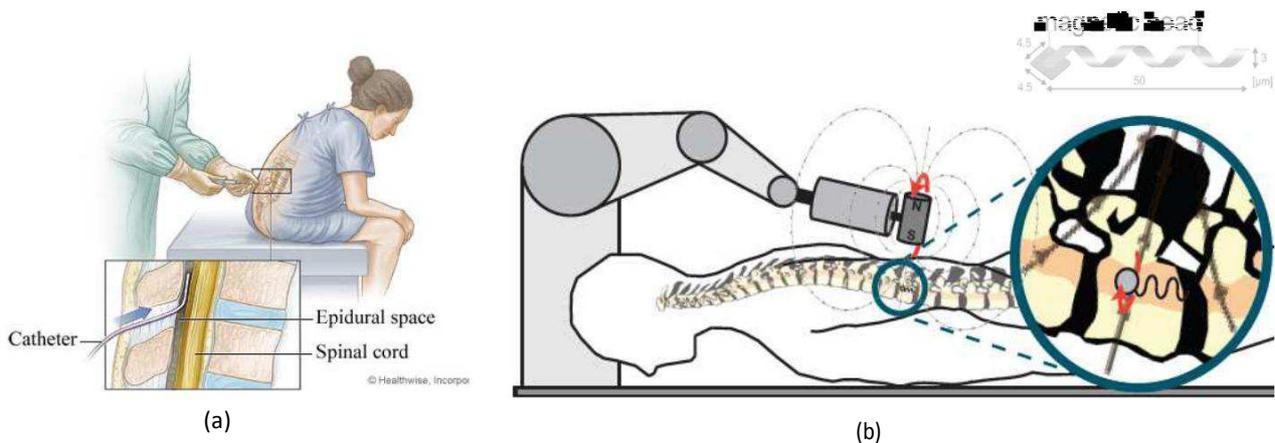
Figure 1: Conceptual images of BMB platform: (a) Injection through a catheter swarms of artificial magnetic microrobots in the epidural space of the spinal canal, and (b) propulsion of the microrobots (inset) through the spinal canal using a multidegree of freedom-magnetic manipulator.
