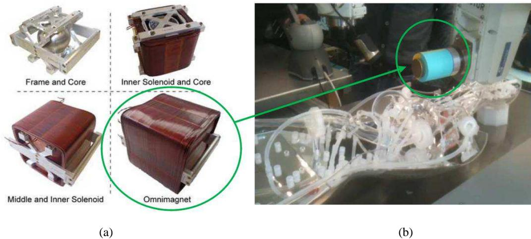
Figure 2. (a) Prototype of 5dof magnetic actuator (Omnimagnet) to be implemented as a robotic end-effector for untethered control of helical magnetic microrobotots and (b) trajectory control along the spinal cord of a human-like phantom model.
